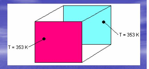
$$c_{\text{loss, conv}} = 2 h_{\text{air}}(T_s - T_{\text{surr}}) = 2 (100 \text{ W/m}^2.\text{K})(80^{\circ}\text{C} - 25^{\circ}\text{C})$$
