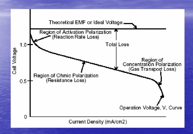
$\Delta G_{\text{max}} = nFE^{\circ} = (2 \text{ electrons } / 1 \text{ mol H}_2)((96,487 \text{ C})(1.229 \text{ V})$ = 237,165 J/mol H<sub>2</sub>
